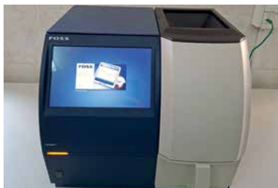
Foss Infratec™ analyser for grain analysis using NIR technology.
