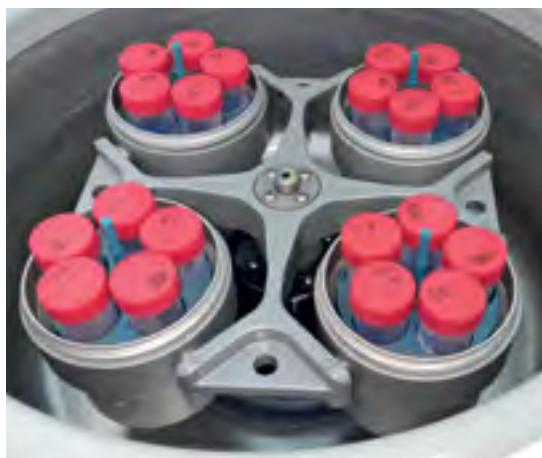
Sample centrifugation – QuEChERS technique.
