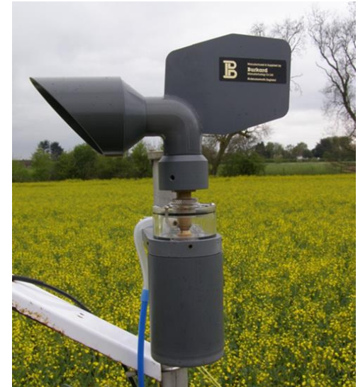
Air sampler (patent) in operation to detect spores of Sclerotinia sclerotiorum
