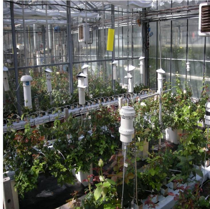
Fig. 1. Temperature and humidity sensors distributions inside the greenhouse compartment.
