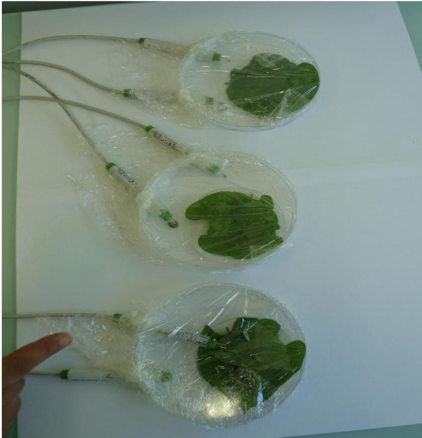
The experimental setup used to measure the microclimate in the domatia and the tissues
