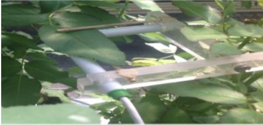
Customized mount bracket of temperature and humidity sensors on the leaf
